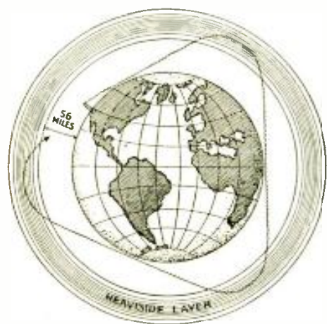
Fig. 1—Short waves are reflected out of the Heaviside layer, 100 km. (56 miles) above the earth, and can thus encircle the earth several times.
