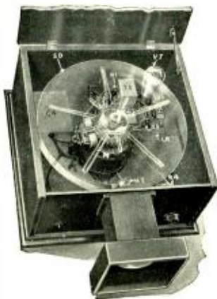
THE COMPLETED TELEVISION UNIT This "X-Ray" picture shows the complete assembly in the cabinet, as if you were looking thru the Scanning Spider.
