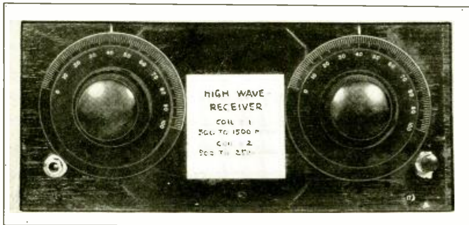
Front panel appearance of Mr. Robbins' "long wave" receiver for listening in above 600 meters. Code as well as European broadcast may be heard.
