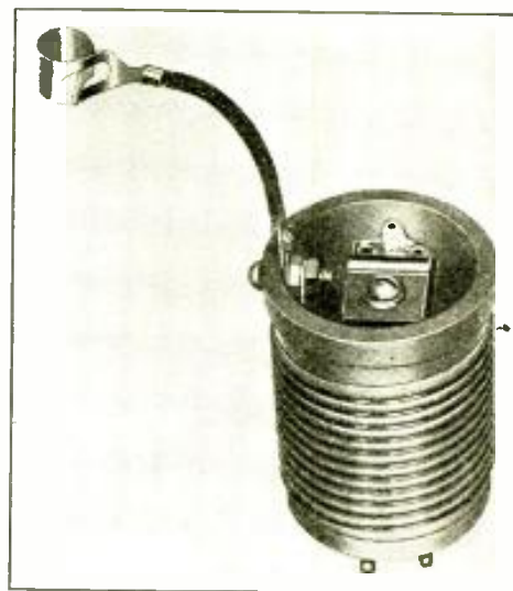
Fig. 5—"Band spreader" coil and condenser for use in "Thrill Box" receiver; makes for easier tuning.
