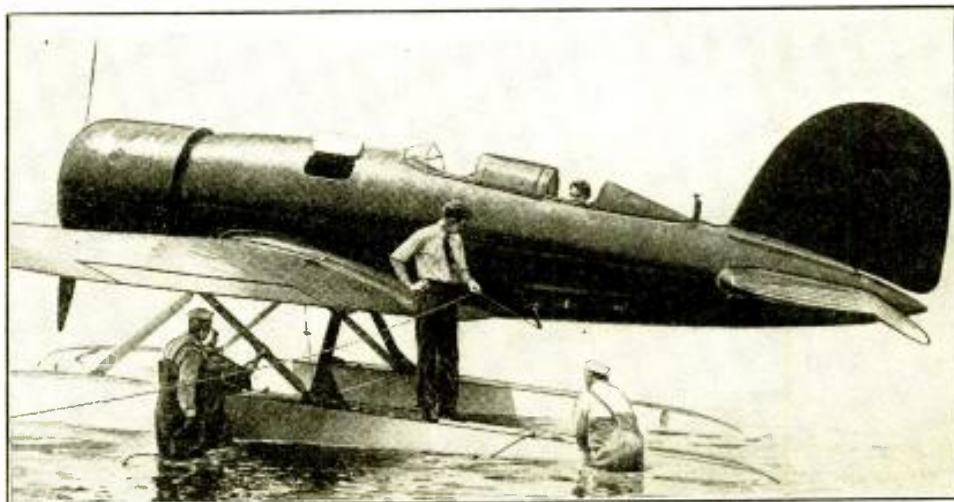
Col. Lindbergh is seen standing on one of the pontoons of his plane (Mrs. Lindbergh seated in the rear cockpit) and he is examining the trailing antenna wire, which is reeled up of course when "taking off." Mrs. Lindbergh operated the radio transmitter and receiver.
