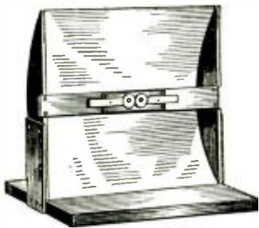
Fig. 3—Spark sender with mirror for decimeter (tenth of a meter) waves.
