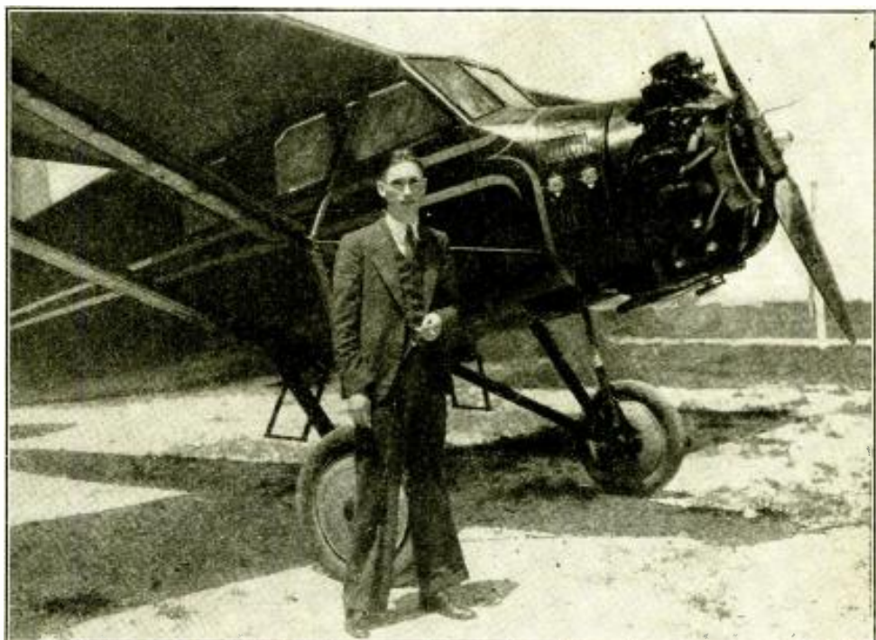
The radio ship, "City of Houston", which was successfully flown and "radio-directed" at the Houston (Texas) municipal airport. Whitney Owen, transport pilot, who went aloft in the plane during the demonstration, is standing in front of the monoplane. The ship remained under the control of a short wave transmitter in the hands of Robert E. Autrey, who manipulated the controls by short wave radio.
