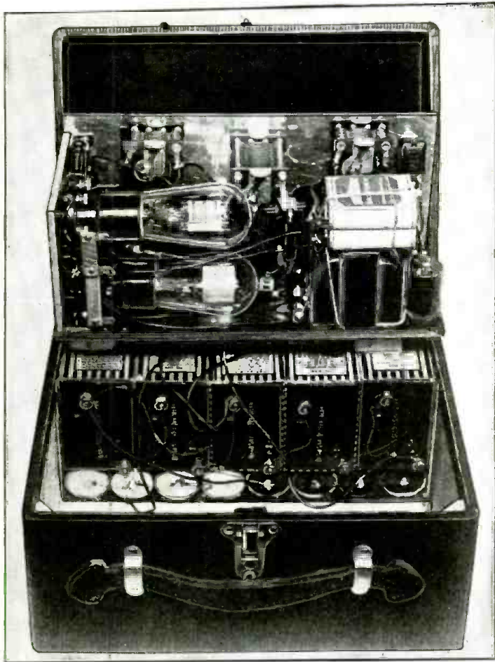
Chassis and battery compartment of "S.W.C." portable.
